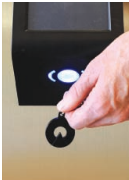
Photo above, top: Rick Flusche, assistant manager — operations, The Crescent. Photo above, bottom: PORT devices can read a variety of identification media, such as ID cards, PIN codes, wristwatches or key rings like the one shown here.
