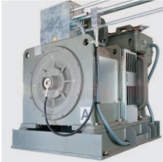
Schindler modular gearless machines are specifically designed to simplify installation in existing machine rooms, while maintaining optimized ride quality. They can be disassembled at the job site and then reassembled in the machine room.
