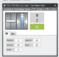
Car status view displays the status of an individual elevator including operation mode, door position, and direction of travel.
