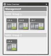
The status overview window shows the elevator and escalator groups, as well as a combined view of all elevators and escalators contained in one building.
