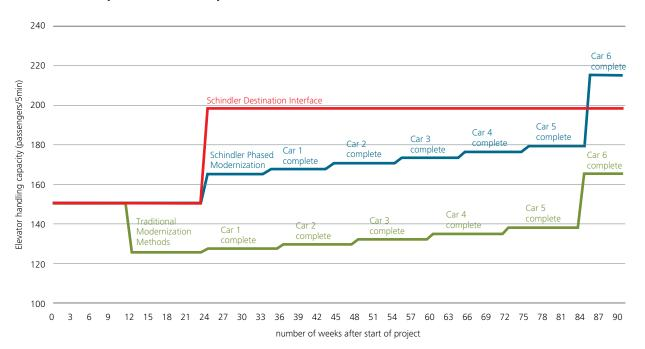
Destination Interface immediately improves system efficiency without taking cars out of service. Phased Modernization provides the same immediate improvement. However, Phased Modernization systems with one car out of service can perform at higher efficiency levels than conventional systems with all cars fully operational.
