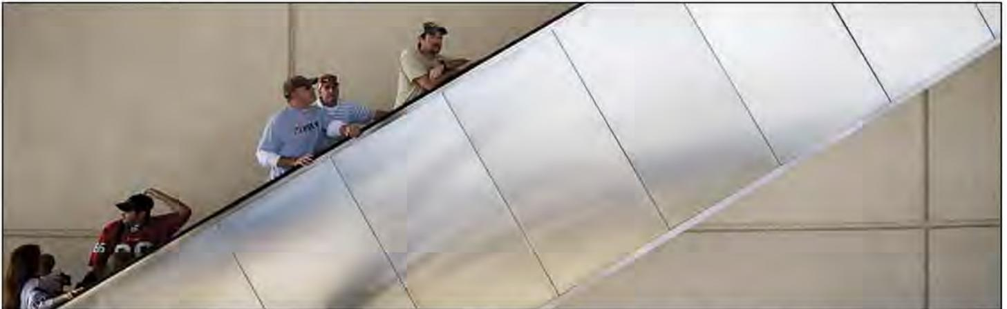
*For high-traffic locations, understanding escalator passenger flow and loading can be complex. Theoretical capacity values may not reflect simple observation or what some studies have shown. Even at peak hours, there are usually empty steps on escalators.*
