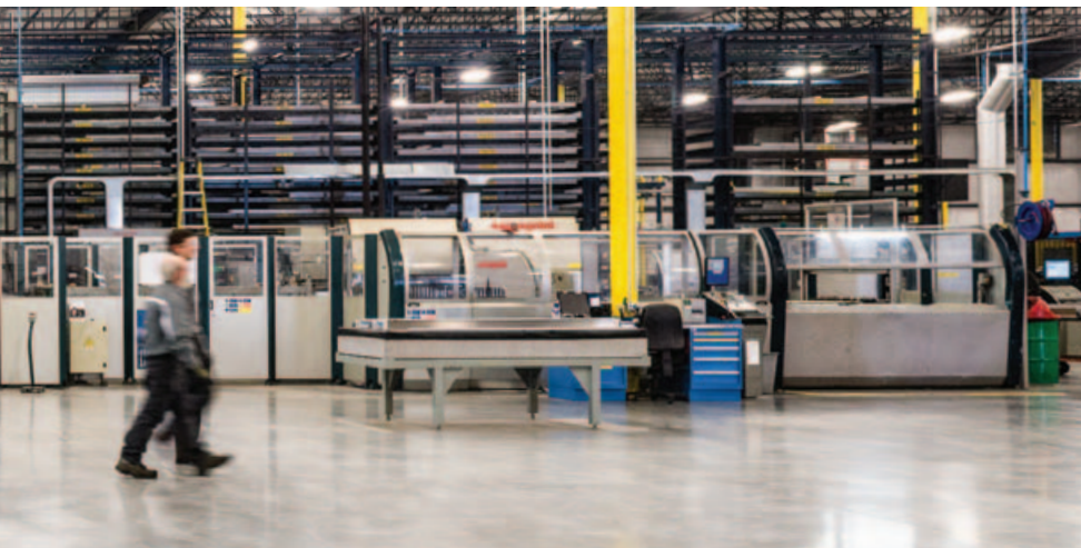
Photo, left: A giant Salvagnini machine fabricates elevator components from flat sheets of metal. Considered a "lean manufacturing tool", the Salvagnini machine reduces manufacturing costs by eliminating waste and has the ability to produce a variety of products in small lots for just-in-time delivery. Photo below, left: The powder coating line brings a colorful finish to elevator parts. Photo below, middle: Photovoltaic solar panels provide half of the Hanover facility's total annual power consumption. Photo below, right: One of the electric car charging stations located at the Schindler Hanover facility.
