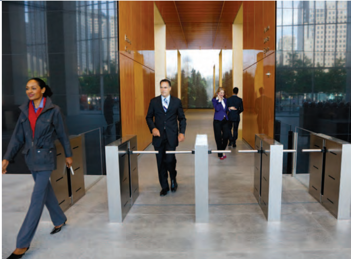
Photo above: Card readers are incorporated into turnstiles to offer tenants personalized service to bring them to their destination floor. Photo below, right: Black granite lobby walls provide a dramatic foreground for the polished African hardwood that leads to the elevator banks.
