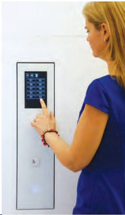
Photo right: Visitors can enter their floor destination at Schindler PORT terminals.
