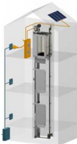
Solar elevator integrated with existing photovoltaics (PV) panel system.
