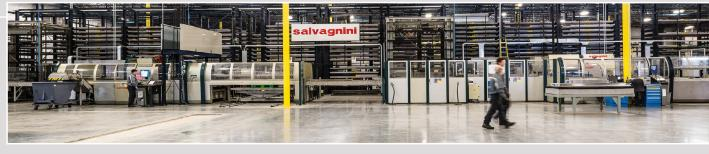
The **high performance, versatile Salvagnini manufacturing system** is designed to punch, shear and bend sheet metal into specialized elevator components with quality and precision.
