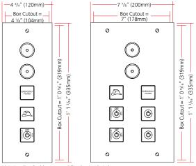
Main Landing Pushbuttons and Fire Service Switch
