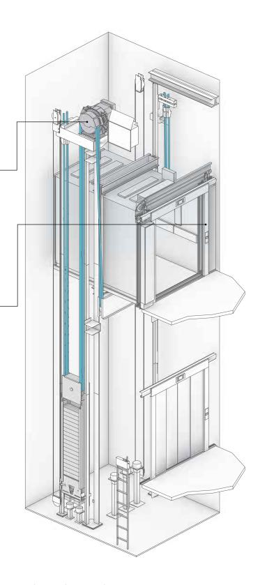
Machine room-less traction elevator
