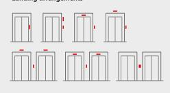
Choose your optimal landing arrangements for simplex and multiplex installations, surface or wall mounting.
