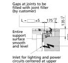
Inlet for lighting and power circuits centered at upper end, through front face
