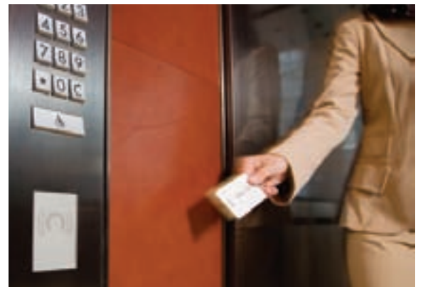
Schindler ID® destination-dispatch system with access control is gaining widespread use for enhanced building security. Passengers identify themselves with a badge, PIN code or other electronically readable device. The system automatically assigns an elevator car that conforms to their approved level of access.
